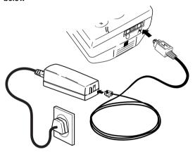
The charging process will start automatically, indicated by a green light on the charger. If the phone is turned off during charging, the LED turns red, and the battery icon flashes sequentially.
